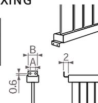
Configurations on size: see parts. Non standard-fixings are welded to the radiator and cannot be changed or reordered afterwards.
